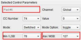
The first press of Pad 6 will send a CC# 74 command with a value of 78, which will close the filter down part way but still let a lot of the audio pass through. The second press of Pad 6 will send a value of 127, opening the filter completely.
