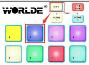
In the picture above the combination of the Shift button and Pad 2 will select Preset #2 from the TUNAMINI preset memory locations.
