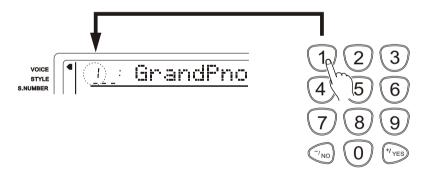
If you want to input large voice number ( $100\sim152$ ), press the NUMBER button 1 till it appears on the first position, and then input the rest two numbers by the way above.
