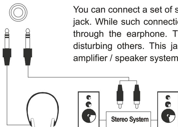
You can connect a set of stereo headphones to the PHONES/OUTPUT jack. While such connection is made, you could only hear the sound through the earphone. Thus, you could practice and play without disturbing others. This jack can also be connected to the external amplifier / speaker system, in order to form a better amplifier system.
