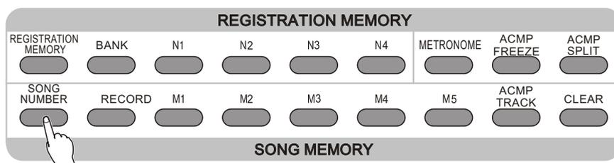
2 Press and hold down the button corresponding to the track to be erased.
