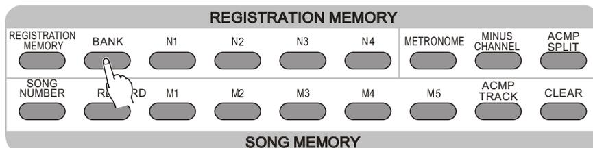
2 Then press the register number you want, and it will be recalled. The register number will be shown in the first line of the screen for a short time and then the original display recovers.
