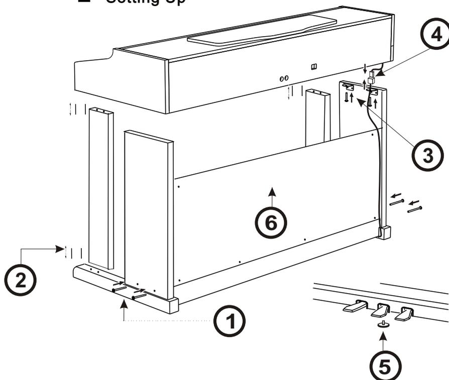
1. Fix the left and right feet on the ground board with 4 black screws at each side.
