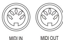
MIDI IN could be used to receive the MIDI data from the outside equipment connected.
